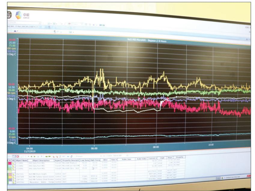
With the bagasse, for example, they were previously only measuring moisture content via moisture meter, whereas now the Micro NIR is providing moisture, pol and fibre every seven seconds.
