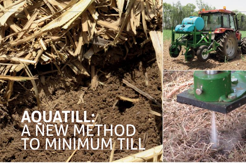
IMPROVED CANE TRASH RETENTION AND THE ABILITY TO TILL IN A WIDE RANGE OF CONDITIONS, GREATER SOIL HEALTH AND MOISTURE CONSERVATION AND REDUCED SOIL EROSION: THIS IS JUST THE BEGINNING OF WHAT A NEW MINIMUM TILLAGE SYSTEM, AQUATILL, MAY BE ABLE TO PROVIDE. BY HANNAH RUSSELL, GRADUATE ADOPTION OFFICER
