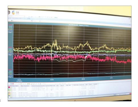
With the bagasse, for example, they were previously only measuring moisture content via moisture meter, whereas now the Micro NIR is providing moisture, pol and fibre every seven seconds.
