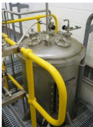
Figure 11 1000 L bioreactor at Mackay Renewable Biocommodities Pilot Plant
