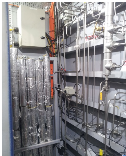
Figure 14 Continuous hydrothermal liquefaction reactor at QUT Banyo Pilot Precinct
