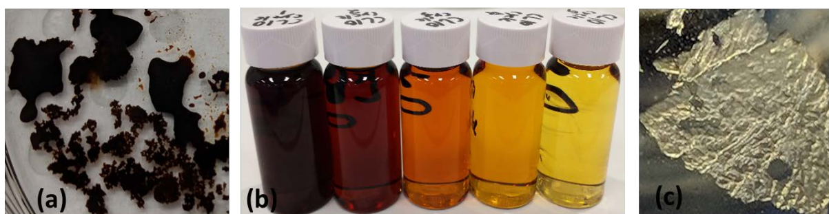
Figure 8 CMF of different purities (a) commercial, (b) different stages of CMF purification, and (c) crystalline
