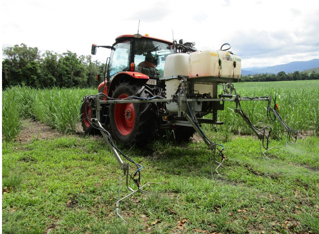
Figure 18: Spraying with the DAF dual herbicide spray bars at Glen Anderson's farm, 2016.
