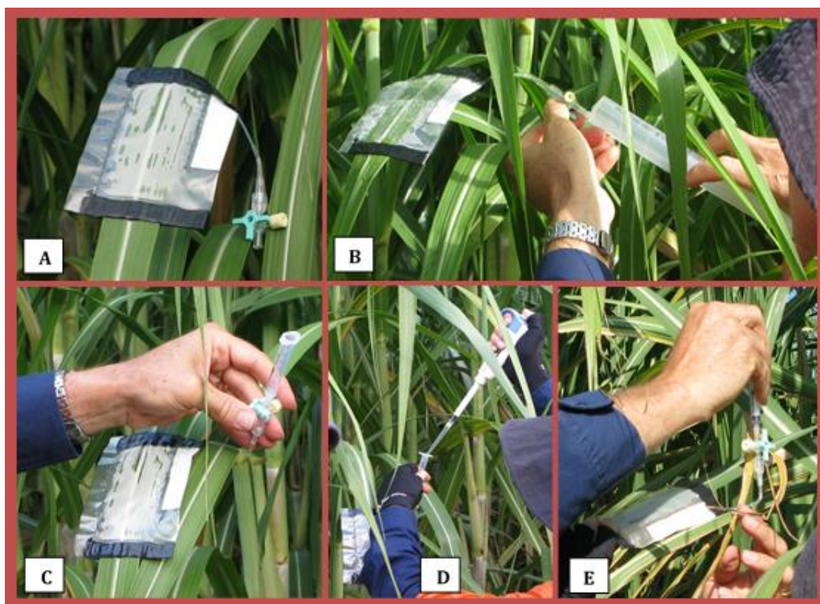
Figure 3 ^{13}\text{C} labelling Q240 ^{\Phi} in field; ^{13}\text{C} delivery chamber (volume: \approx 100\text{mL} ) plastic acetate sheet heat sealed to form a chamber 124 x 80 mm with two 12 mm strips of Consolidated Alloys Butyl rubber sealant at each end (Bunnings part # 10266). The chamber has an internal pocket 70 x 25 mm containing a strip of TOM organic ultra-thin absorbent liner 70 x 20mm. Inserted on top of the liner is a 1.0mm \varnothing x 100mm clear transmission tube attached to a BD blunt end plastic cannula (303345) and Terumo Terufusion 3-way Stopcock Luer Lock (TE-TSWSR201) (A); evacuating chamber and filling with \text{CO}_2 free air (B); addition of \text{NaH}^{13}\text{CO}_3 + HCl and injection into chamber (C-E)
