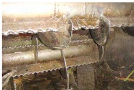
Forward feed components - knockdown roller and finned roller
