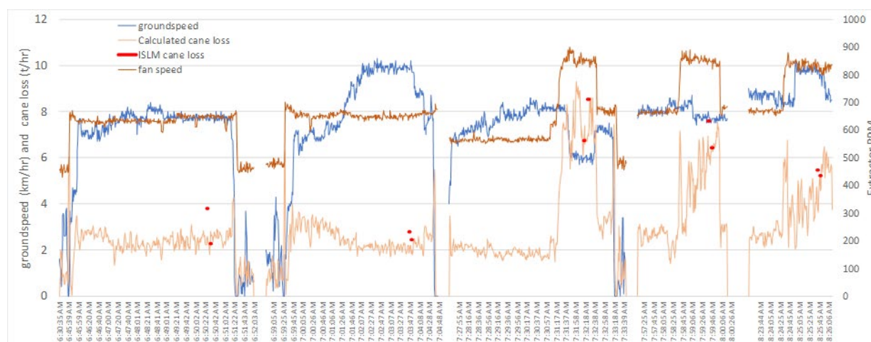
Figure 23. Sample of fan speed and derived cane loss at Ingham showing SCHLOT-estimated cane loss (continuous blue line) against ISLMS cane loss, the latter indicated by the red line at the time the harvester passed the ground sheets that collected cane loss and trash. (Fan speed and Chopper pressure included for reference).
