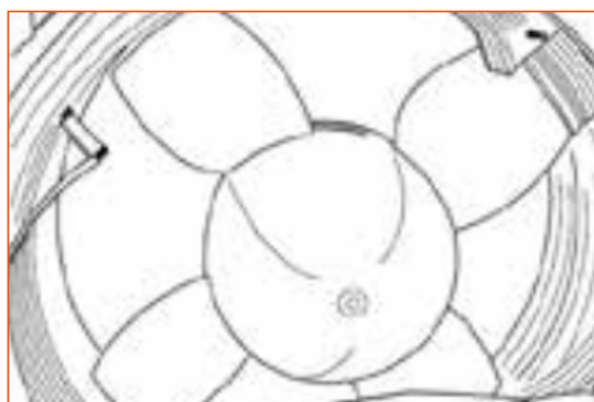
Primary extractor fan – looking upwards inside hood
