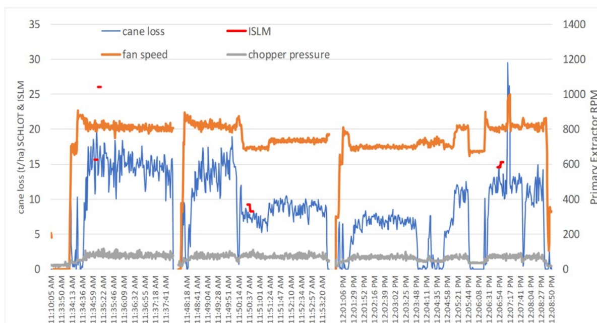
Figure 22. Sample of fan speed and derived cane loss at Rocky Point showing SCHLOT-estimated cane loss (continuous blue line) against ISLMS cane loss, the latter indicated by the red line at the time the harvester passed the ground sheets that collected cane loss and trash. (Fan speed and Chopper pressure included for reference)
