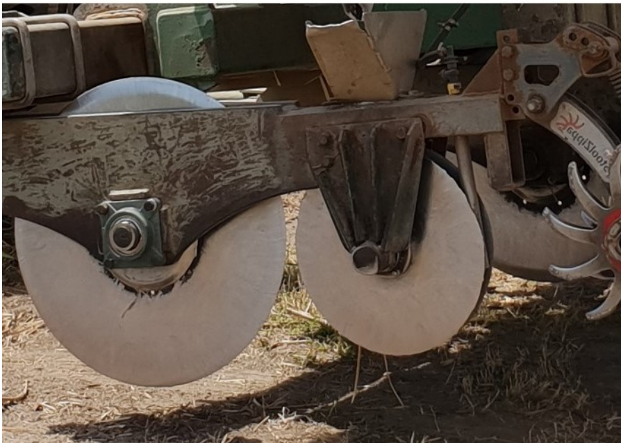
Images 22 and 23: Examples of poor alignment of the delivery nozzle
