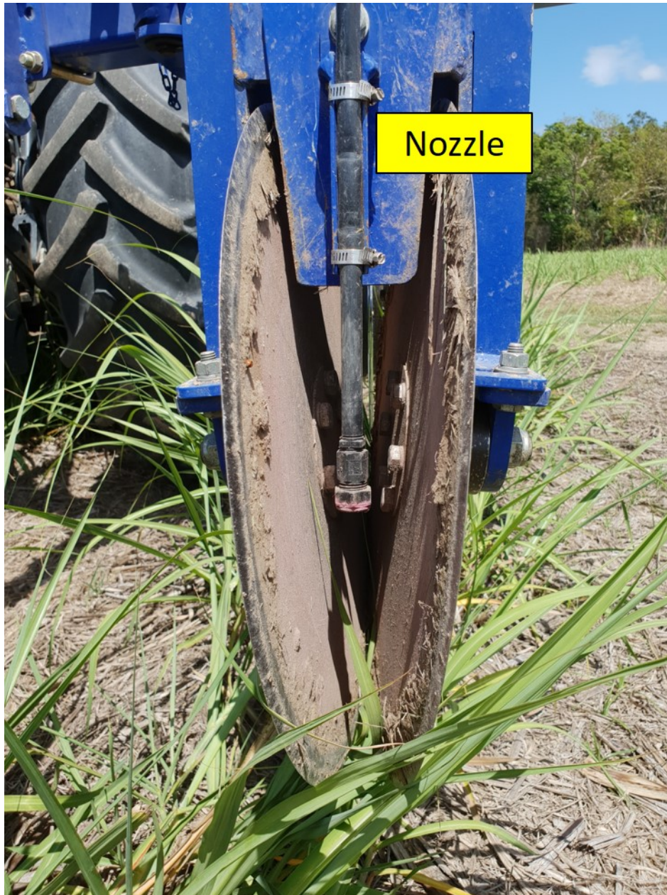
Image 1: Delivery nozzle located between double discs
