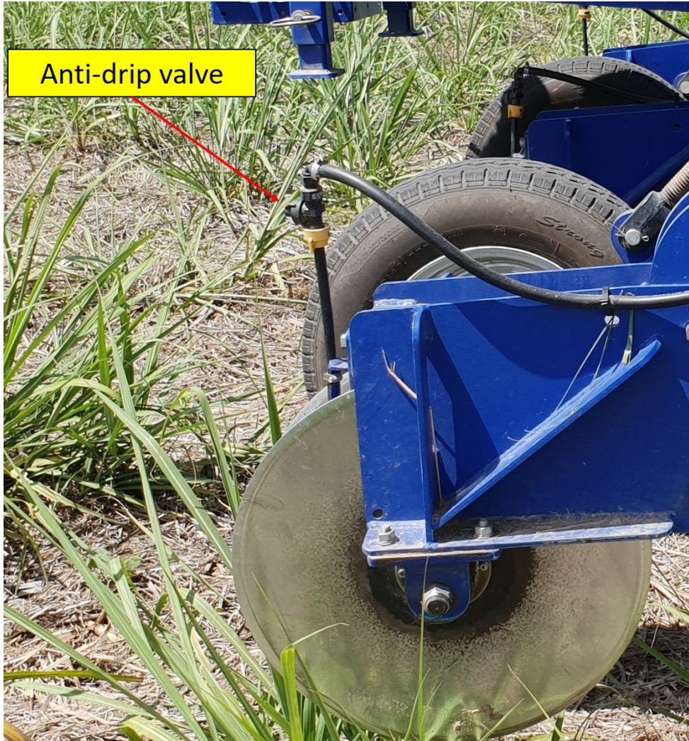
Image 34: Anti-drip valve located on delivery line
