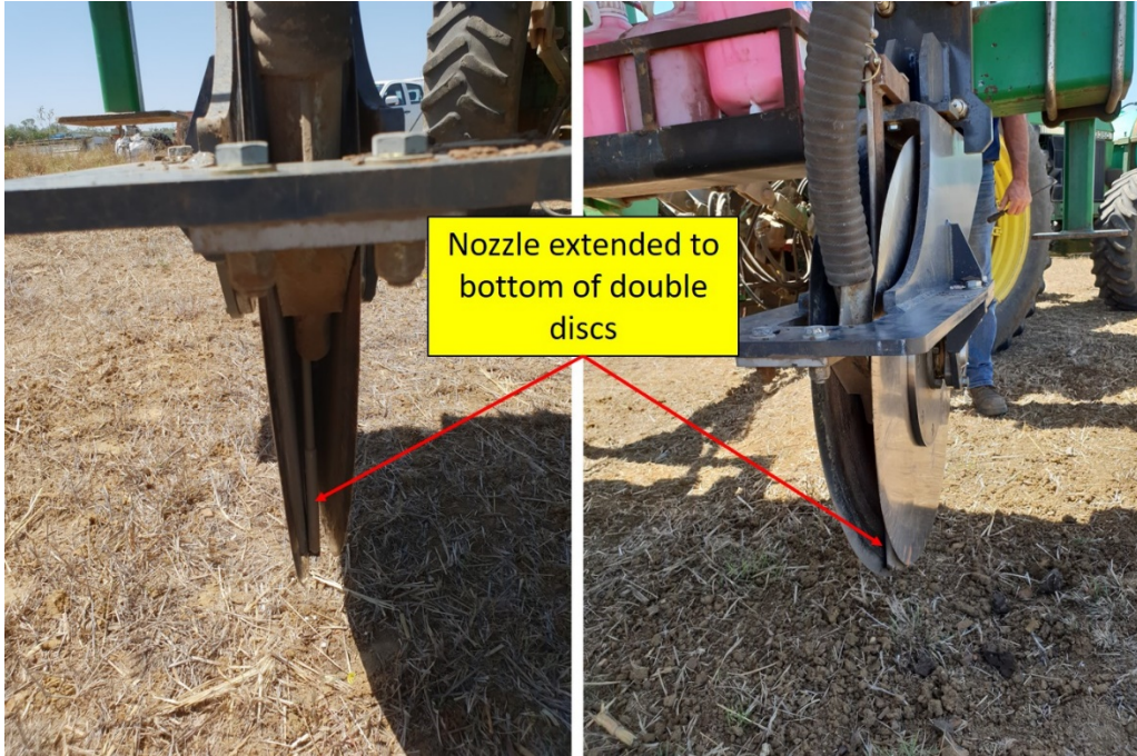
Images 18 and 19: Nozzle extended to bottom of slot in double disc opener arrangement
