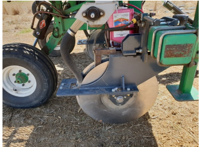
Images 5 and 6: Examples of double disc only applicators, that-is no leading coulers
