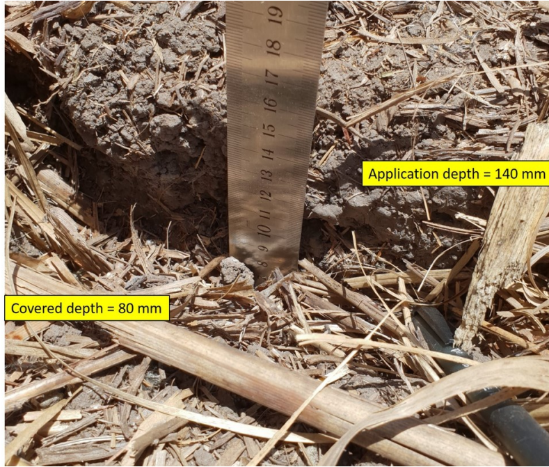
Image 36: Example #2 of imidacloprid applicator assessment field measurements
