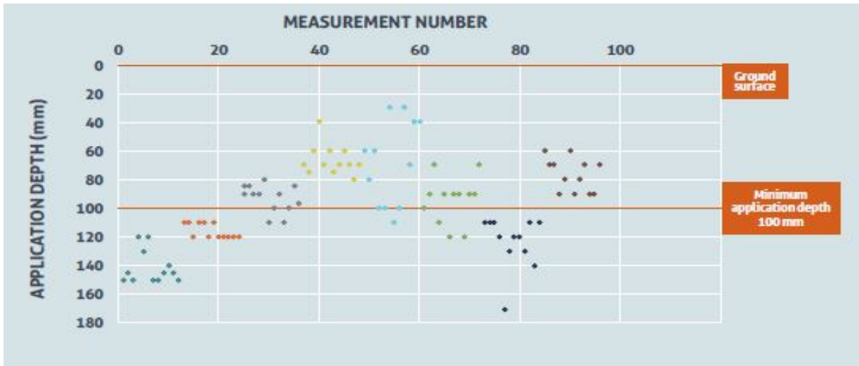
Figure 1: Measured application depths for eight double disc opener units in the Herbert. Fifty percent of measurements were less than 100 mm.
