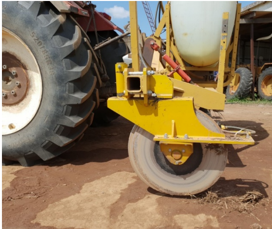
Images 5 and 6: Examples of double disc only applicators, that-is no leading coulers
