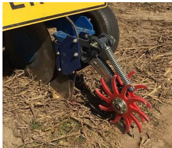
Figure 2. StoolZippa™ behind a stool-splitter tine assembly.
