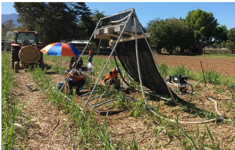
Figure 3. Rainfall simulator and small field plot.
