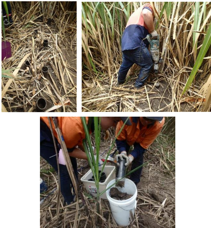
Figure 2. Field collection of root samples: Top left - placement of cores; Top right - inserting cores using jackhammer; Bottom - emptying out the cores.
