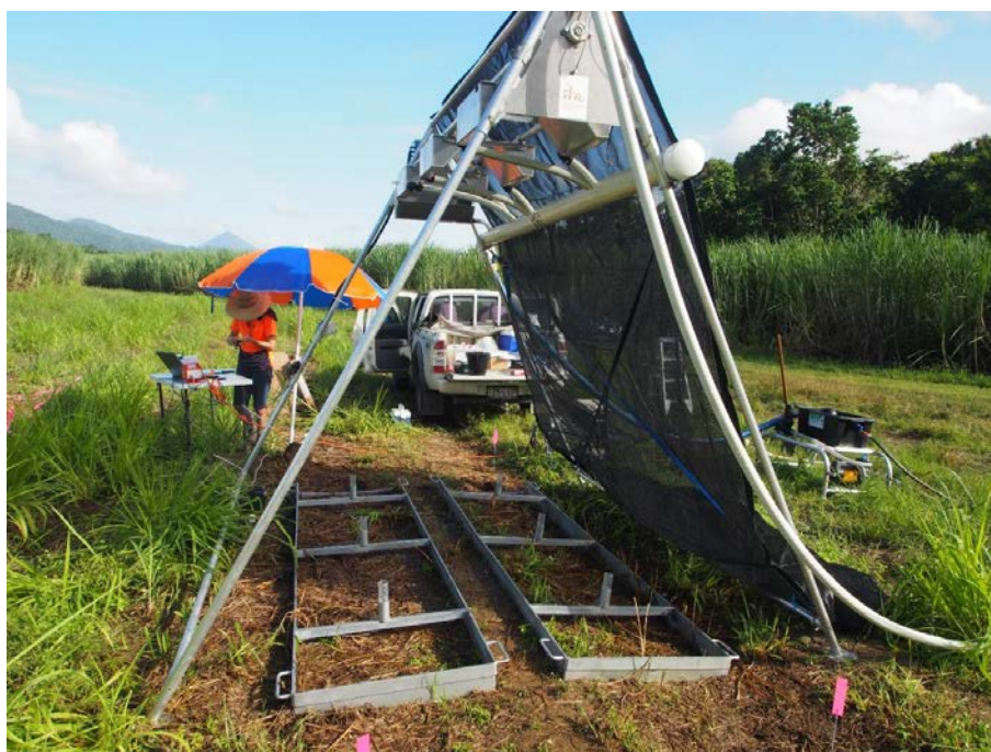
Fig. 1—SRA Rainfall simulator installed on replicate 1 (Mix 1 was applied to the left plot, Mix 2 was applied to the right plot).
