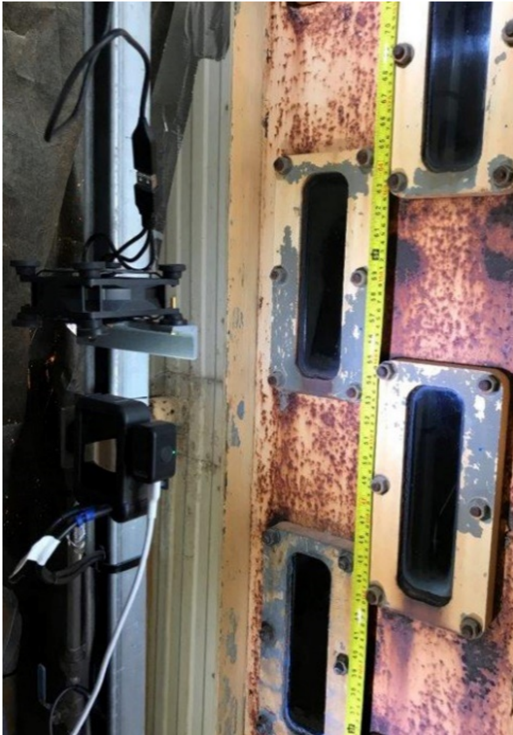
Figure 8 Measuring tape to allow calibration of the images
