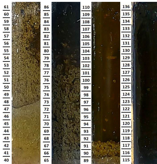
Figure 22 Images from VPMS showing pocket of juice on 22.11.2020 at 00:19
