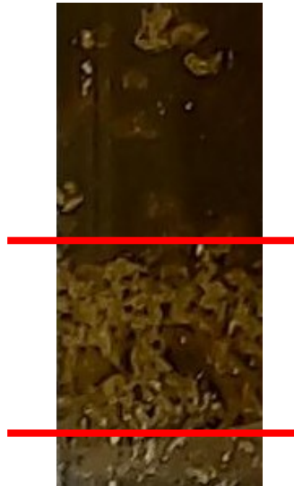
Figure 15 Mud settlement in a clarifier showing three distinct regions
