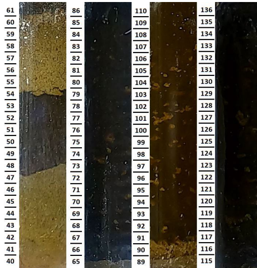
Figure 21 Images from VPMS showing detached block of mud solids on 18.11.2020 at 00:00
