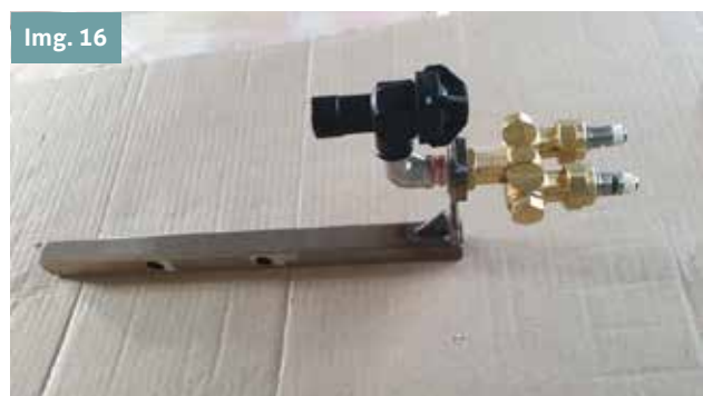
Image 15 and 16: Farmacist, Project Bluewater Case Studies Directed Herbicide Spray in Sugarcane and Floodjet® Nozzles.
