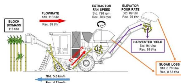
**Figure 1.** Differences in speeds, flow rate, sugar loss, pour rate and cane yield between standard (Std.) and recommended (Rec.) practices.
