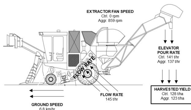
**Figure 3:** Differences in fan speed, pour rate and cane yield between aggressive (Aggr.) and Control (Ctrl.) treatments.
