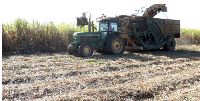
Measuring cane yield with commercial harvesters and weighing equipment. Sucrose and fibre content are analysed by Near Infrared Spectroscopy (NIR).
