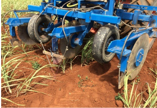
Figure 4 Nuprid applicator set up in plant cane
