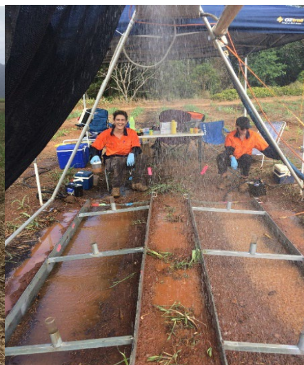
Figure 16 Rainfall simulation at trial RH5
