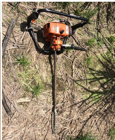
Figure 9 Petrol auger for soil sampling at trial IF1
