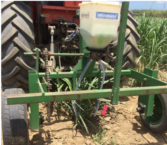
Figure 6 suSCon applicator in plant cane
