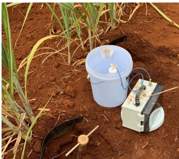
Figure 10 Prenart suction cup installation at trial IF3
