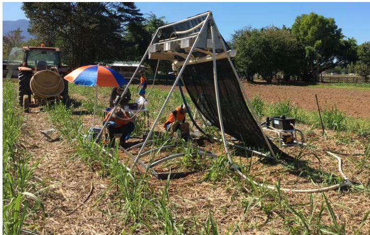
Figure 13 Rainfall simulator and quadrat, trial IP1.
