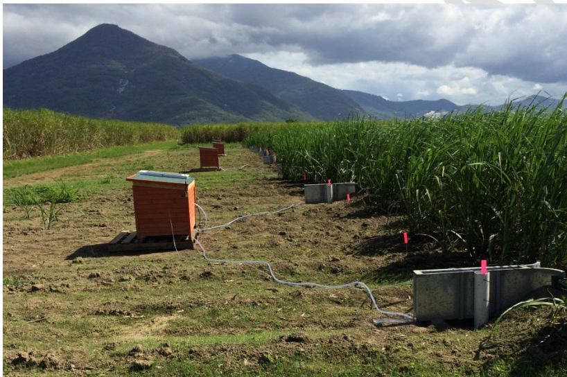
Figure 7 Flumes with stilling wells, suction and bubbler lines and wooden boxes containing ISCO samplers, loggers, telemetry and batteries at trial IF1, 2017
