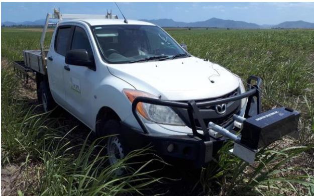
Figure 1a: Radiation Solutions RS-700 (Radiation Solutions, Mississauga, Ontario, Canada) and RSX-1 detector.
