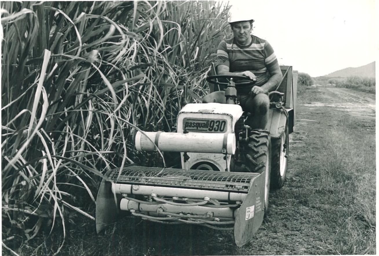
The front-mounted inter-row rope-wick applicator with shrouds in 'normal' operating position.
