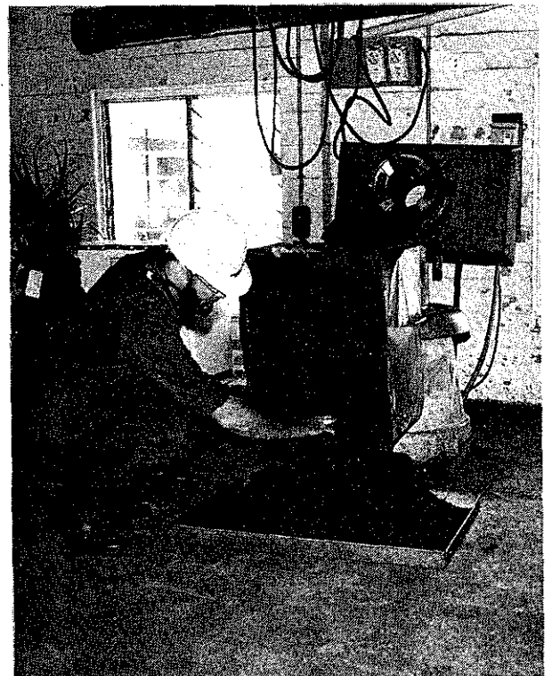
PLATE 4 - Removing hammer milled leaf material from cutter-grinder prior to sampling for moisture, fibre and wet disintegrator sub-samples
