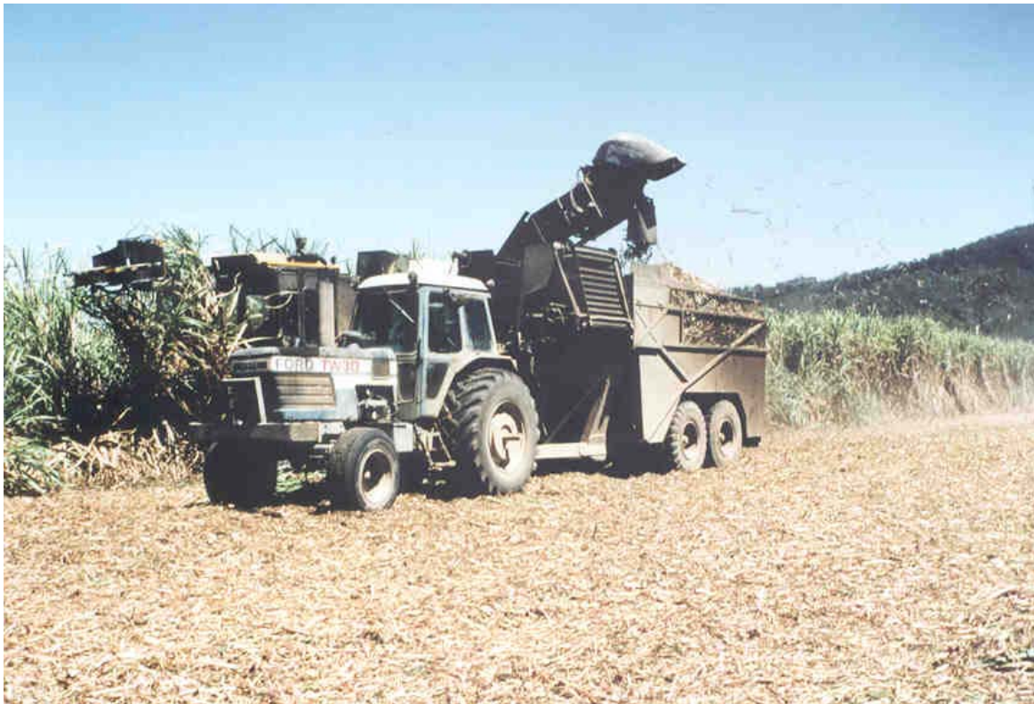
Figure 1: Large haulout equipment used in the sugar industry. What is the cost due to soil compaction?
