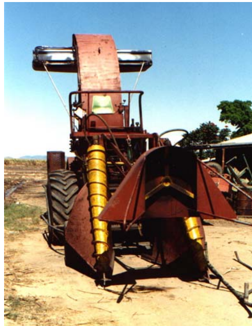
Plate 3 - Cannavan single row, chop throw harvester without a blower cleaning system fitted
