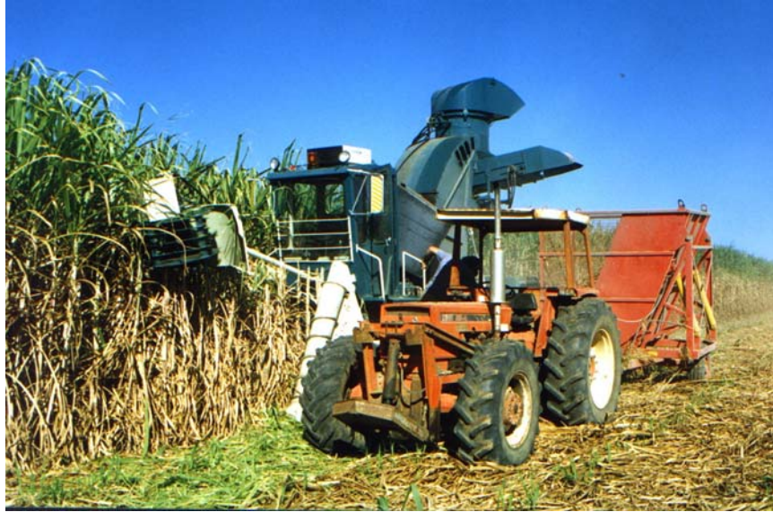
Plate 6 - The 1996 Bonel single row, chop-throw harvester fitted with an extractor cleaning system at the front of the thrower chute, just above the thrower
