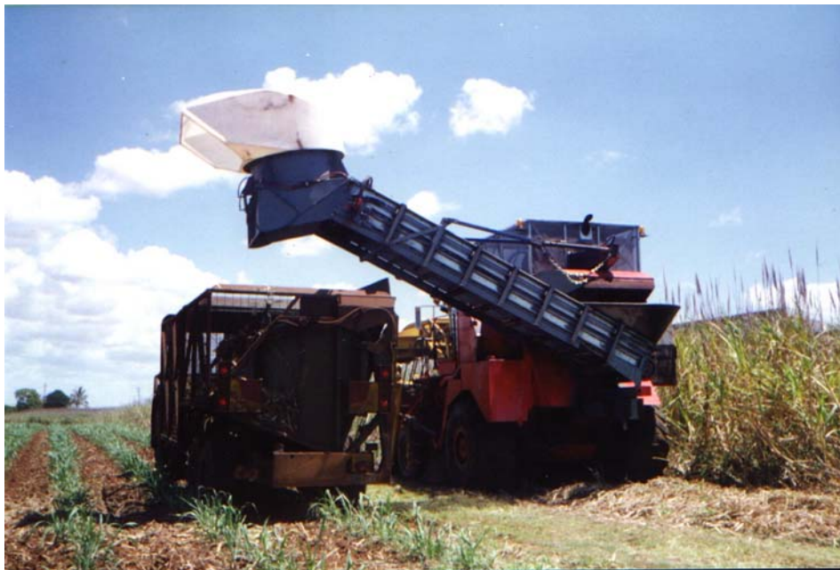
Plate 2 - Rear view of the Young two row, chop throw harvester showing the outlets of the twin blower cleaning system
