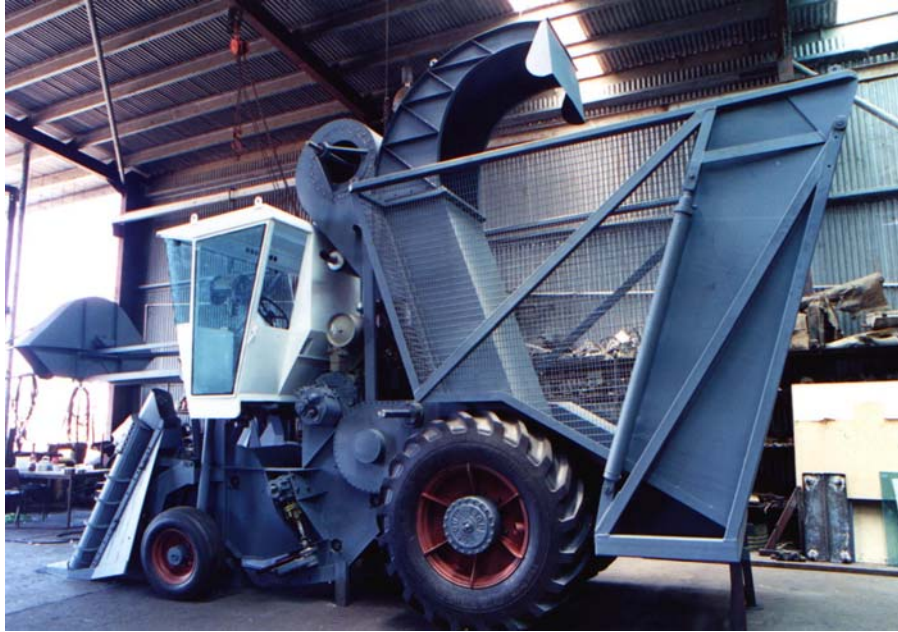
Plate 4 - The 1993 Bonel single row, chop-throw harvester, constructed in the Burdekin by R Gendrolius, and fitted with a blower cleaning system
