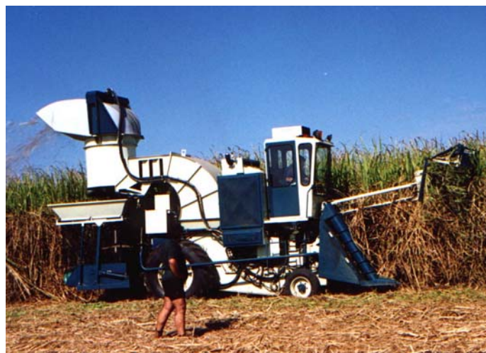
Plate 5 - The 1994 Bonel single row, chop-throw harvester fitted with an extractor cleaning system at the top of the thrower
