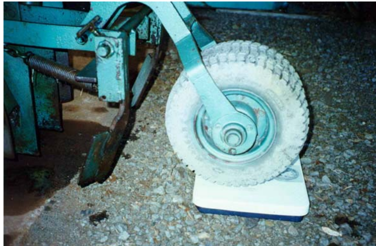
Photo 4 - A wholestalk planter presswheel – note small wheel diameter and the use of bathroom scales for measuring pressing force
