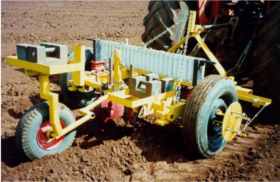
Photo 1 - Magazine planter and presswheel configuration developed for field trials
