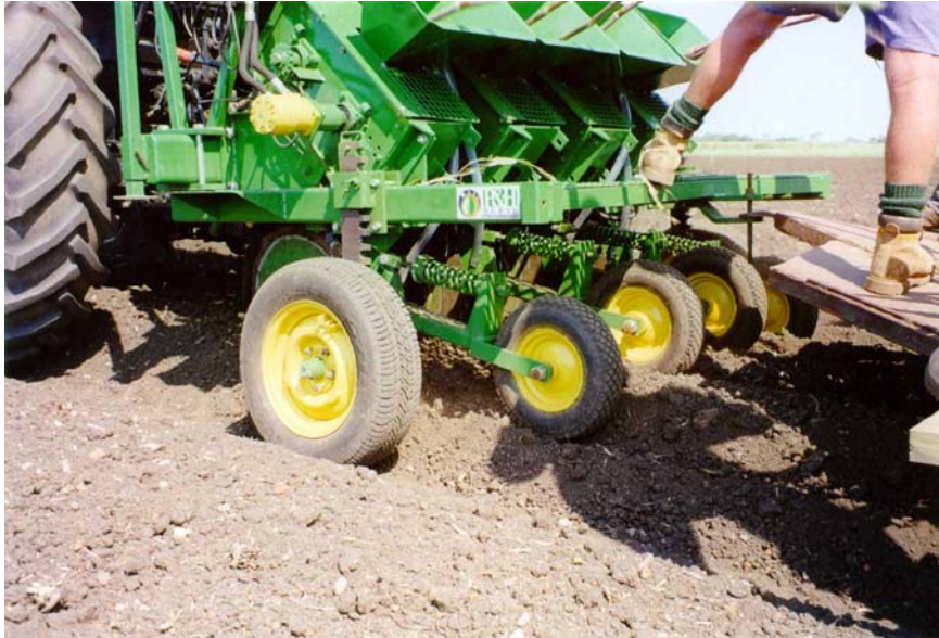
Photo 11 - Presswheel design used on HDP planter – note large diameter wheel
