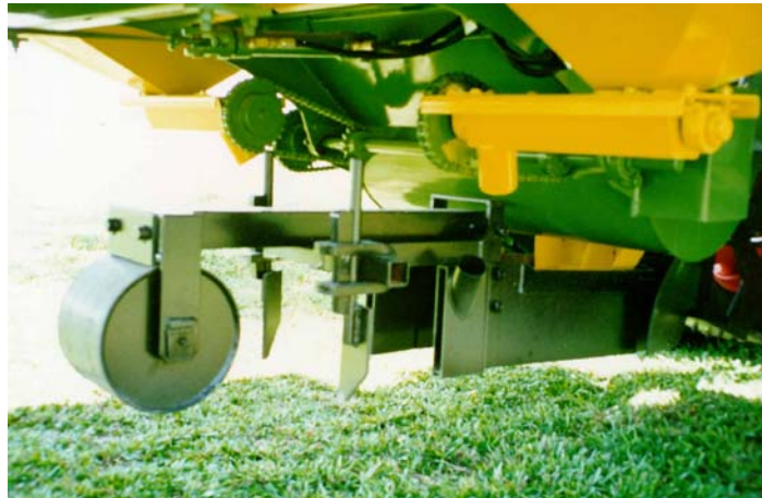
Photo 5 - Steel presswheel used on billet planter – note small diameter solid wheel and lack of spring loading system
