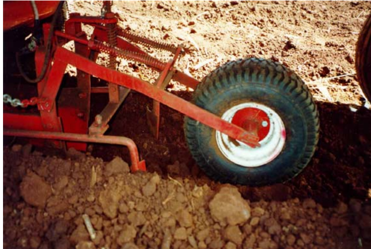
Photo 3 - Commercial sugarcane planter presswheel – note small diameter wheel, light springs, poor spring pre-load adjustment and basic pivots
