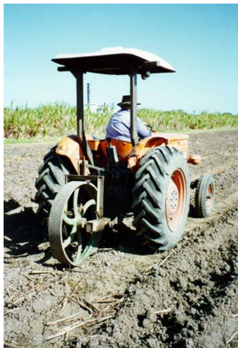
Photo 7 - Cast iron wheel (surplus drive pulley) used as a presswheel at Harwood Mill plantation, NSW
