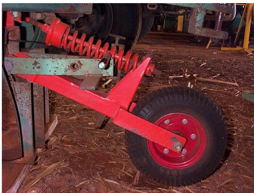
Photo 10 – Presswheel designed during this project retro-fitted to wholestalk planter
