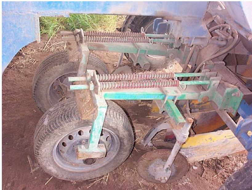
Photo 12 - Robust presswheel designed to suit commercial dual row planter
