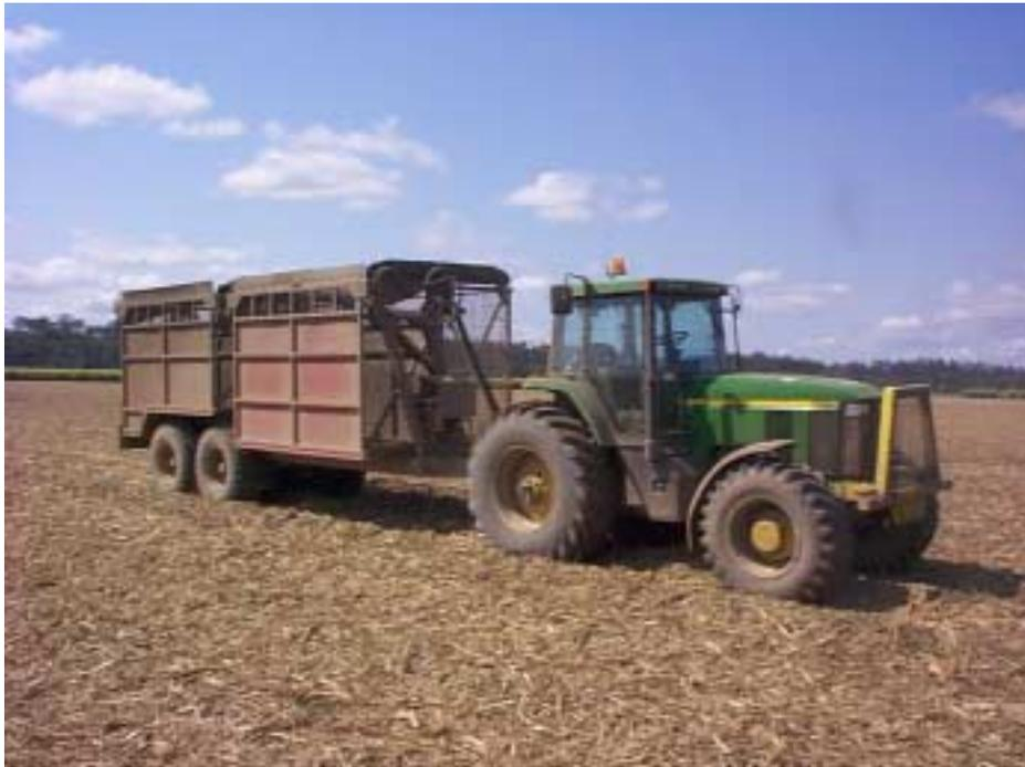
**Figure 13 - John Deere 7810 with 12t LG Engineering trailed bin**
