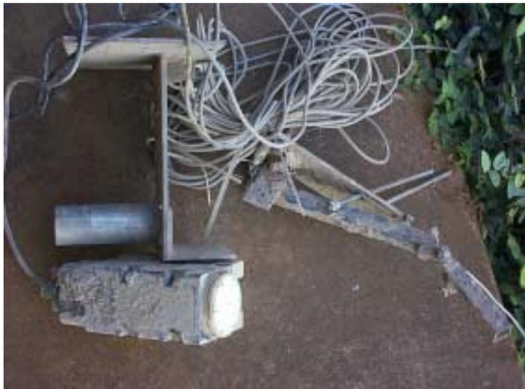
**Figure 10 - Radar and infrared temperature sensor**
