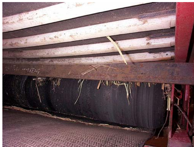
Figure 4: Sagged backing plate and support ribs.
