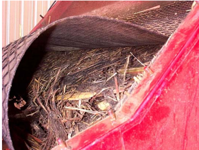
Figure 6: The foreign matter buildup between the bottom roller and belt.
