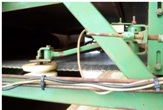
Figure 8: Nylon belt position feedback guide.
