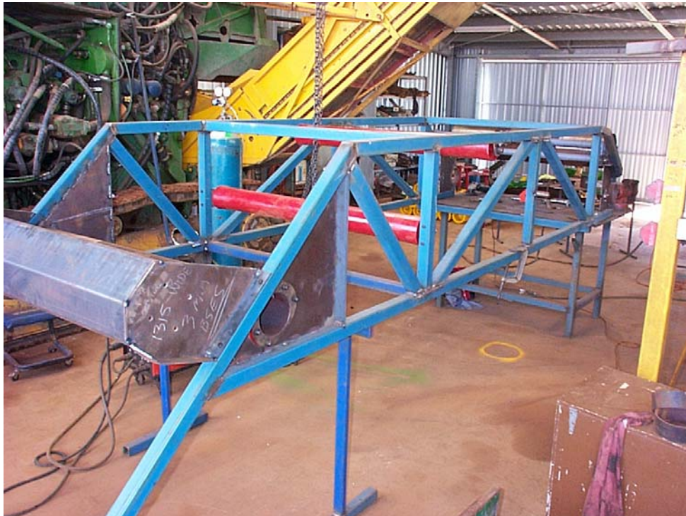
Figure 9: Hugger belt open truss frame during construction.
