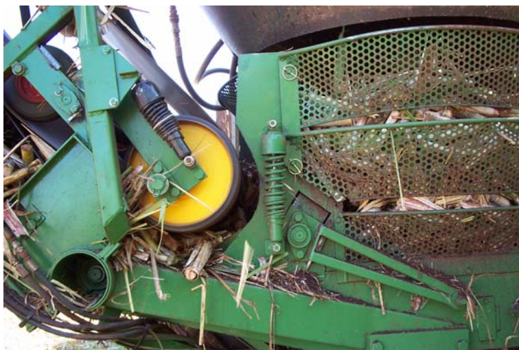
Figure 22: Hugger belt entry system with single large diameter tail roller.
