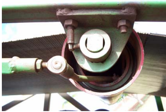
Figure 7: Self-steering roller connected to tactile guidance system.
