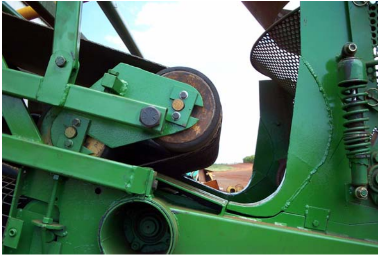
Figure 23: Reconfigured entry geometry of the hugger belt system incorporating twin tail roller arrangement.
