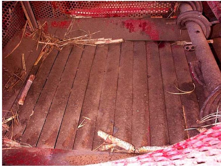
Figure 1: Chain and slat conveyor and spiral wrapped feed roller arrangement.
