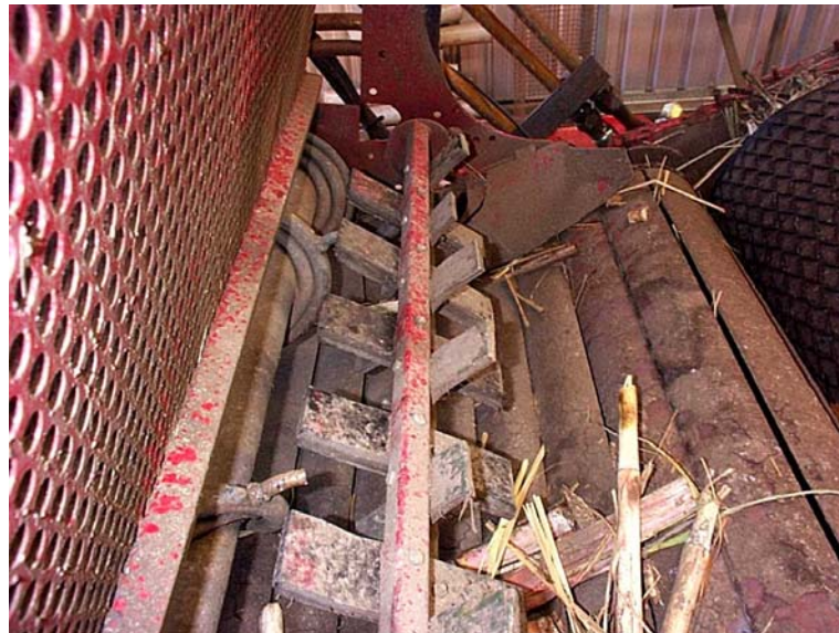
Figure 2: Transition zone of chain and slat conveyor and scalper feed roller arrangement.
