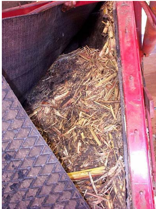
Figure 5: Trash, dirt and whole billet buildup between the bottom belt and the backing plate.
