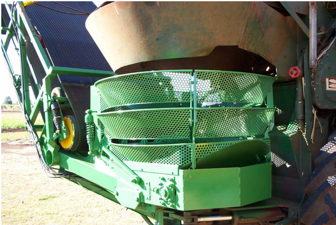
Figure 13: Primary elevator bowl and turntable arrangement.
