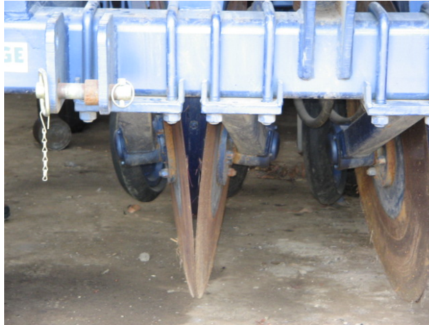
Figure 5 Double discs utilised as a furrow opener during planting
