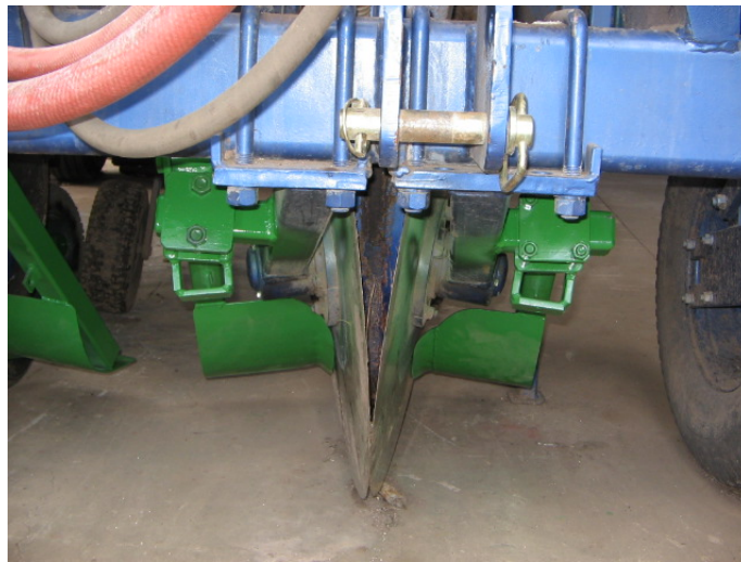
Figure 6 Disc-scraper modification at Rocky Point
