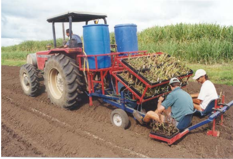
Figure 3 Planting cane with seedling planter
