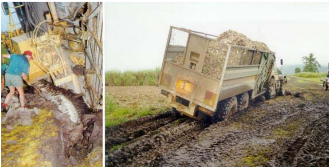
Figure 1: Bogged machinery during the 1998 harvest season that devastated the Australian sugar industry due to excessive rainfall during the later half of the harvest season. Industry was unable to harvest all of the sugarcane, and in attempting to do so severely damaged the ground and impeded crop growth for future ratoons. The technique outlined in Everingham et al. (2008) would have provided an early warning about the threat of harvest rainfall if it had been operational during 1998. Starting the harvest season earlier, harvesting lower lying paddocks earlier and with greater urgency could have saved industry many millions of dollars.
