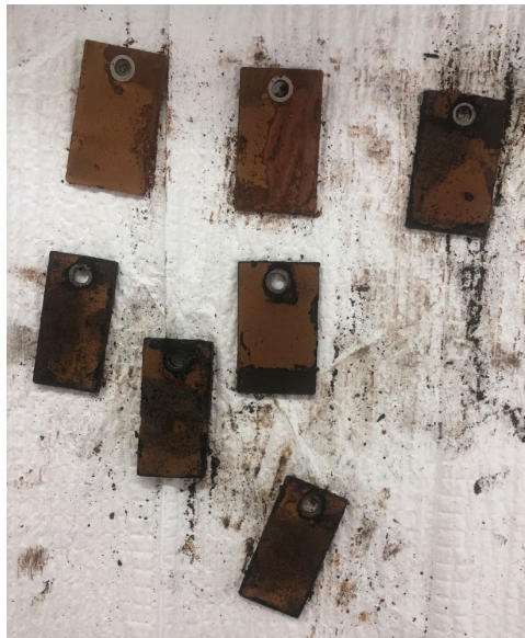
Figure 10 30-day corroded coupons at Invicta Mill.
