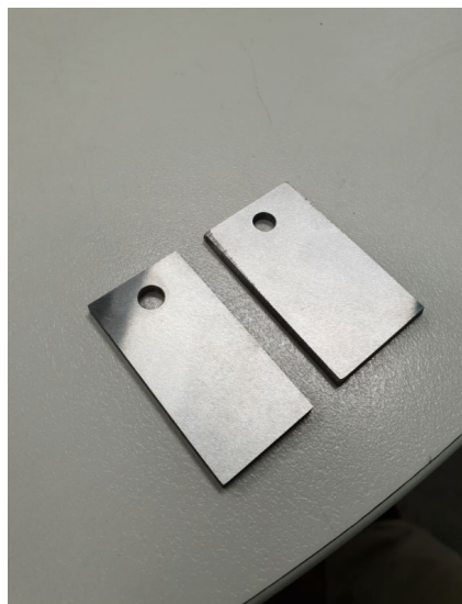
Figure 4 Example of coupon surface finish to avoid excessive corrosion caused by surface defects.
