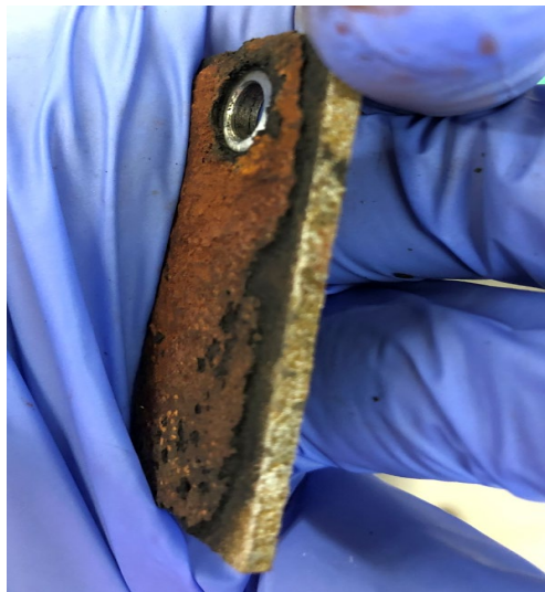
Figure 11 60-day corroded tube plate coupon at Invicta.
