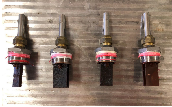
Figure 9 30-day corroded coupons at Isis Mill.
