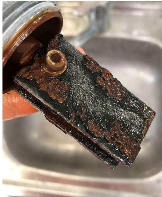
Figure 14 Tube plate material coupons corroded at Invicta Mill by 60 days of exposure to final condensate.
